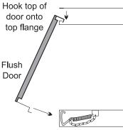
Be careful that the glass gasket does not roll up; there must be a gap between the gasket and the door lip to ensure that the door sits securely on the unit. Diagram 2.
